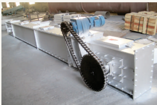
High Temperature dust-proof housing that can also be gas Tight
